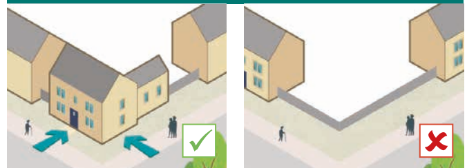
Buildings should be located where two routes meet and positively address both sides with doors and/or windows
